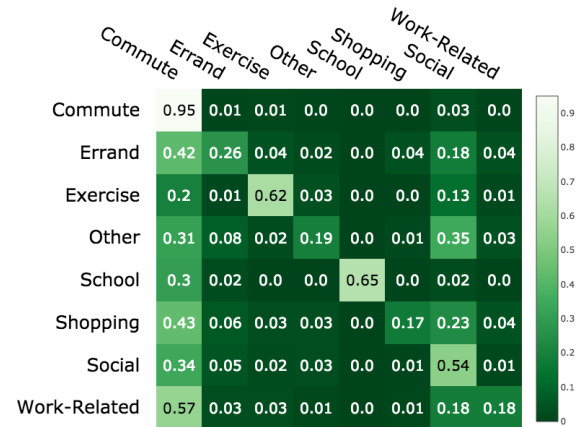
Fig. 6. Confusion Matrix for XGBoost with eight classes. Darker colors represent best trip purpose classification values. Most of the classification errors wrongly assign as trip purpose either commute or social as can be observed in those two columns and rows.
